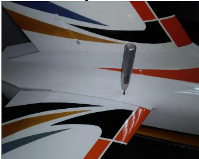
44. Fix the stab to fuselage with screws.
