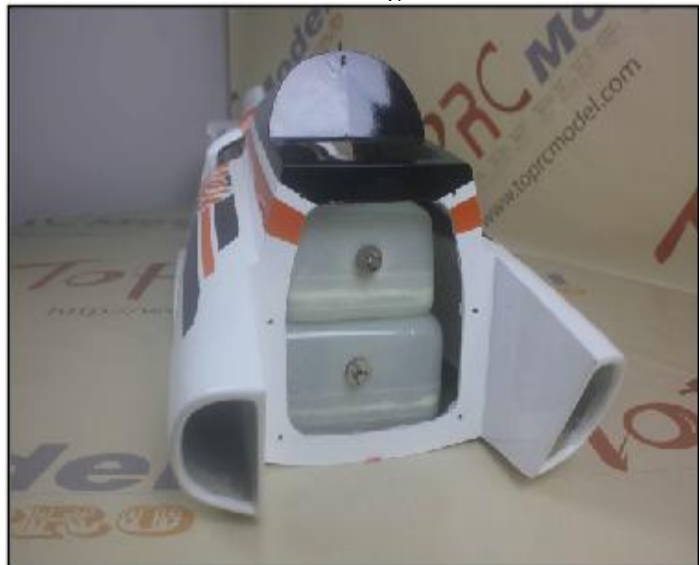
27. Put the fuel tanks in the fuselage.
