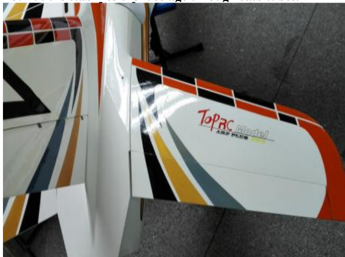
43. Put the stab into the fuselage through stab tubes.
