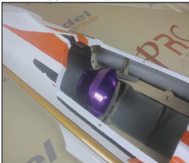
29. Fix the tail pipe to the fuselage with screws.
