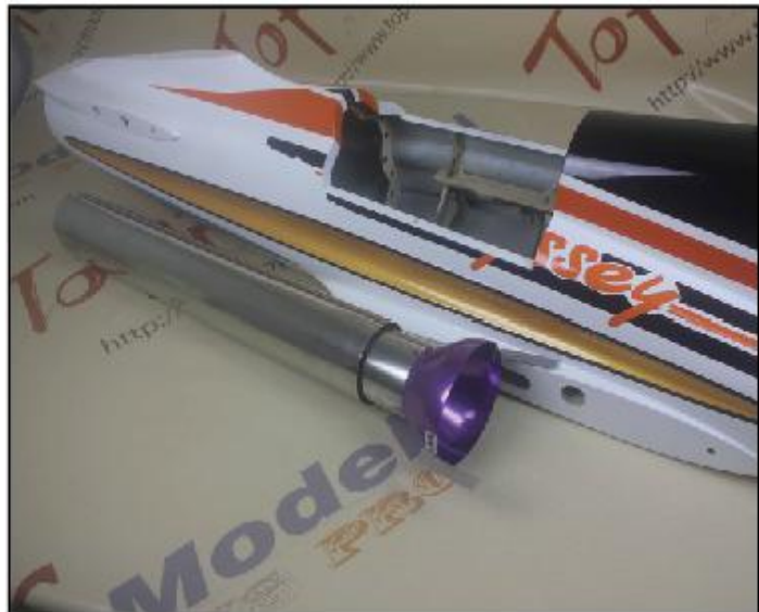
28. Put the tail pipe to the fuselage.
