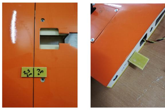
*Glue the fiberglass' 2,5cm part on the wing. Use sandpaper on the fiberglas for better glue result.*
