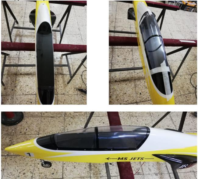
Cut the canopy to fix, while the base part screwed on the fuselage. Use Patex soft glue (or similar). Also use 8pcs 2,5 x 12mm screws - included in the kit.
