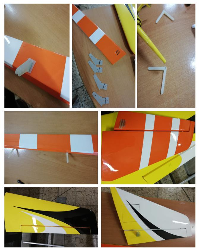
Cut the oracover for flap hinges and use epoxy glue. Use sandpaper on the horn parts for better glue result.
