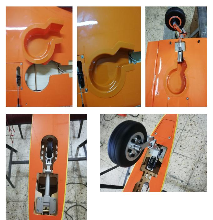
Stick the plastic pools to the mid-wing with epoxy glue, than screw the retracts with 12pcs 3 x 20mm screws included in the kit.
