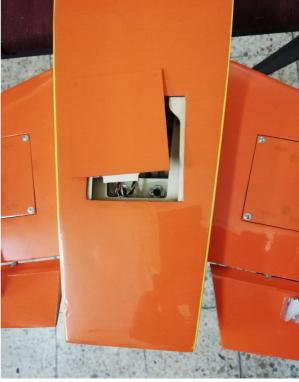
Mark the fiberglass parts on each stabilizer and drill a 4mm hole for fixing.
