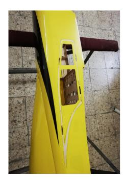
Use epoxy glue to assemble fiberglass intake
