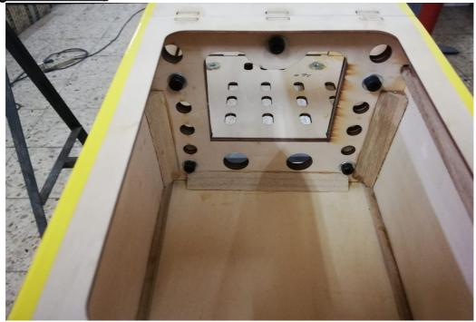
Install front part to main fuselage part by using 5pcs 5  $\times$  25mm Allen screw (included in the kit).
