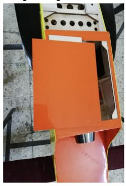
Assemble the engine to front end as close as possible to balance the CG for less extra weight in the nose.
