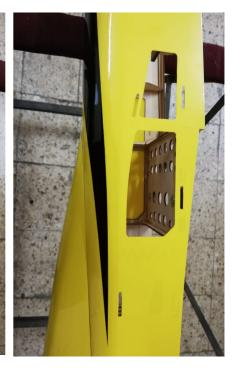
Mark the fiberglass on the fuselage.
