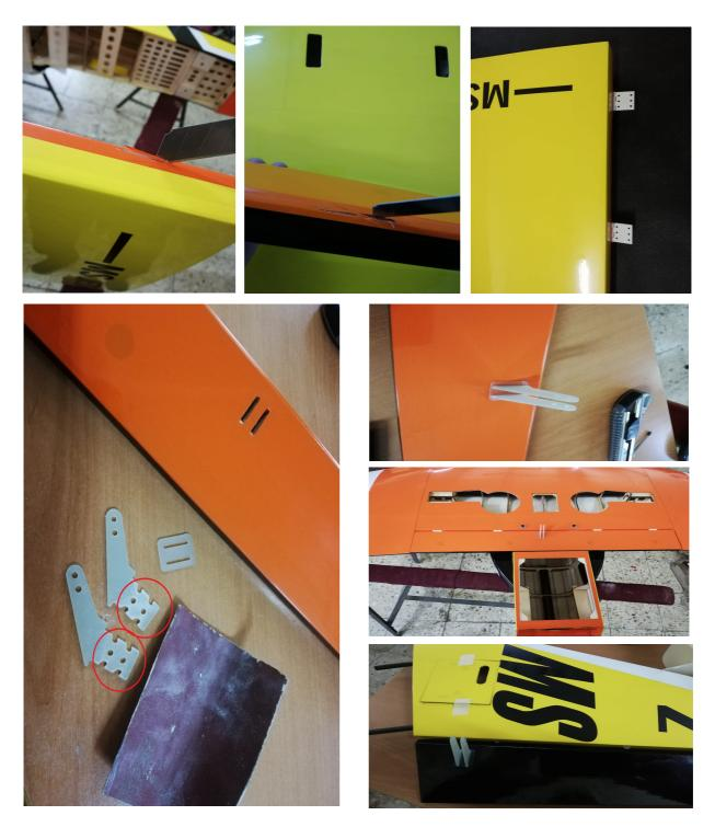
Cut the oracover for flap hinges and use epoxy glue. Use sandpaper on the horn parts for better glue result.
